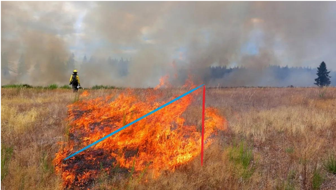
Figure 1. Flame Length measurement scheme. Red line indicates Flame Height and Blue line indicates Flame Length
